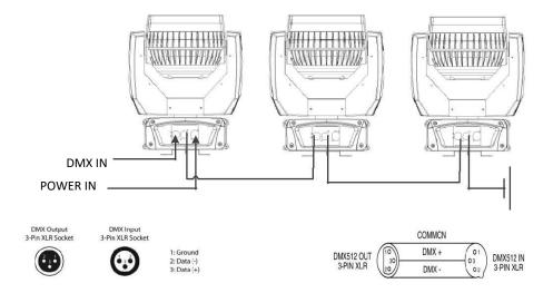
For installations where the DMX cable has to run a long distance or is in an electrically noisy environment, such as in a discotheque, it is recommended to use a DMX terminator. This helps in preventing corruption of the digital control signal by electrical noise. The DMX terminator is simply an XLR plug with a 120  $\Omega$  resistor connected between pins 2 and 3,which is then plugged into the output XLR socket of the last fixture in the chain. Please see illustrations below.
