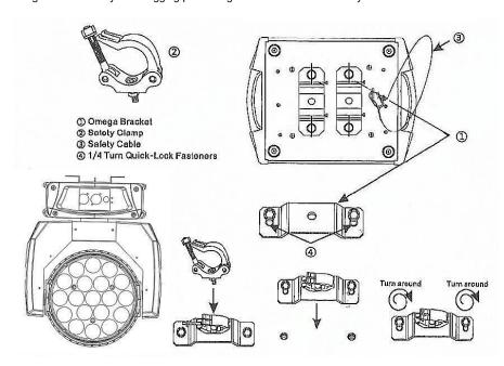
Regardless of the rigging option you choose for your products, always be sure to secure your fixture with a safety cable. The fixture provides a built-in rigging point for a safety cable on the hanging bracket as illustrated above. Be sure to only use the designated rigging point for the safety cable and never secure a safety cable to a carrying handle.
