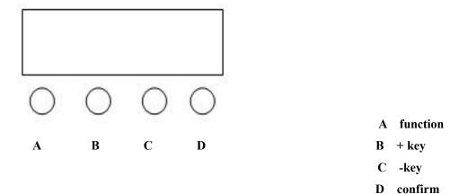
Operation instructions: press the function key, A will cycle out 11 different function effects. The first two digits of the digital tube represent the current function (refer to the function table). The last two digits represent the address code of that function. Or the parameter of the speed. Press the B or C key to modify its parameter values. Press the D key to confirm.
