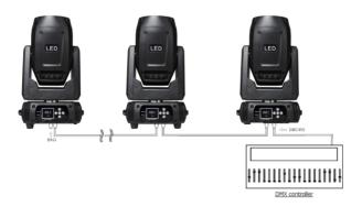
Connect the DMX-output of the first fixture in the DMX-chain with the DMX-input of the next fixture. Always connect one output with the input of the next fixture until all fixtures are connected. Up to 32 fixtures can be connected.
